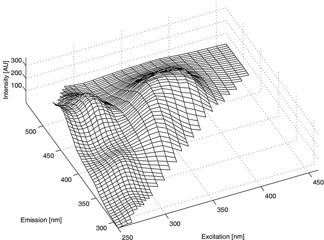
Fig. 5. An example of a fluorescence landscape from HPLC fraction no. 9 (22–23.5 min) of thick juice measured with 31 excitation wavelengths (230–460 nm) and 431 emission wavelengths (288–700 nm). The blank regions hold Rayleigh scatter signals and are thus treated as missing values.
