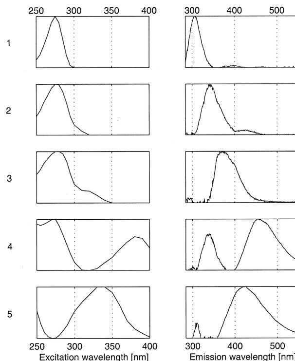
Fig. 2. A five-component CP model of fluorescence landscapes of 10 thick juice samples. The left column shows the resolved excitation profiles and the right column shows the resolved emission profiles of the five components. All profiles have been normalised to unit length.
