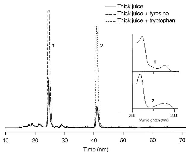
Fig. 3. HPLC size exclusion chromatograms with qualitative standard additions of tyrosine (1) and tryptophan (2) to thick juice monitored by fluorescence detection at 285/325 nm. The chromatograms verify the expected presence of tyrosine and tryptophan. The corresponding UV/VIS absorbance spectra from the diode array scans of the two peaks are also displayed.
