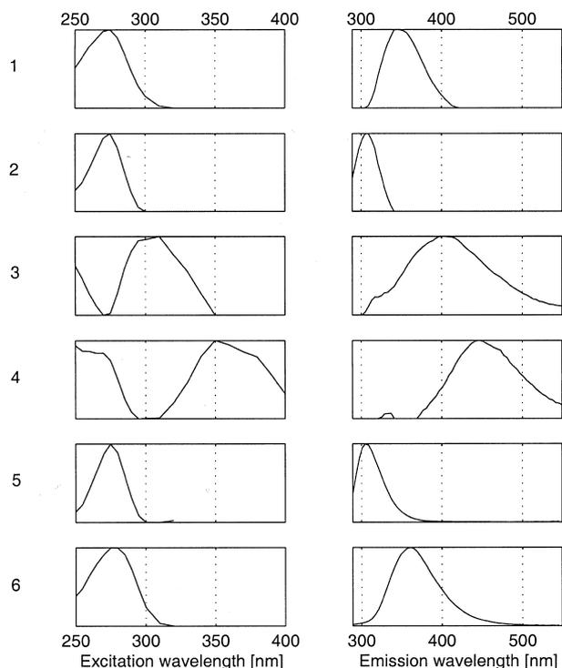
Fig. 1. The results of a four-component CP model of fluorescence landscapes of five beet sugar samples. Rows 1–4 contain the excitation and emission spectra of the four resolved components. The left column shows the excitation profiles and the right column shows the emission profiles. Rows 5 and 6 show the fluorescence excitation and emission spectra of pure tyrosine and pure tryptophan, respectively, for a comparison. All profiles have been normalised to unit length.
