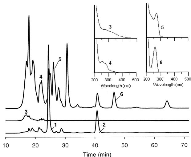
Fig. 4. HPLC size exclusion chromatograms of a thick juice sample. Upper curve: UV detection at 280 nm; middle curve: UV detection at 420 nm; bottom curve: fluorescence detection at 280/325 nm. Diode-array spectra of selected peaks (3–6) are also displayed. The spectra of peaks 1 and 2 are identical with the spectra of the corresponding tyrosine and tryptophan peaks in Fig. 3.
