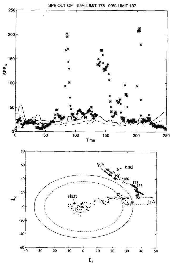
Figure 5 On-line monitoring of batch 56, using multiway PLS: a, squared prediction error; b, progression of batch as projected on second and third latent variables
