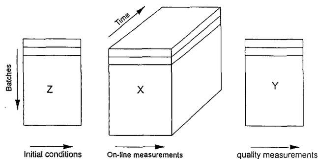
**Figure 1** Nature of the batch data bases. Trajectories of variables in batch process,  $\mathbf{X}$ ; initial conditions or data from pre-processing conditions,  $\mathbf{Z}$ ; quality data,  $\mathbf{Y}$ .
