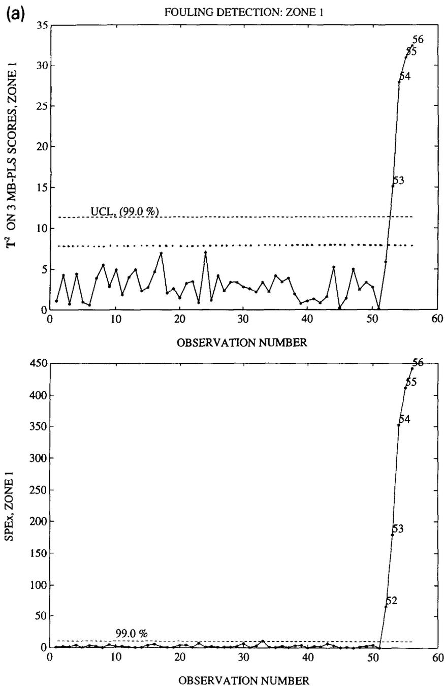
Fig. 6. Monitoring the LDPE process using multi-block PLS. The disturbance is fouling in zone 1. Monitoring of individual zones detects the problematic zone. (a)  $T^2$  chart on three MB-PLS scores and  $SPE_x$  for the process variables of zone 1. (b)  $T^2$  chart on three MB-PLS scores and  $SPE_x$  for the process variables of zone 2.
