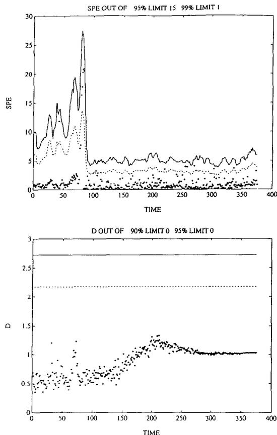
Fig. 9. Monitoring a good batch.  $SPE_x$  and  $D$  statistic.
