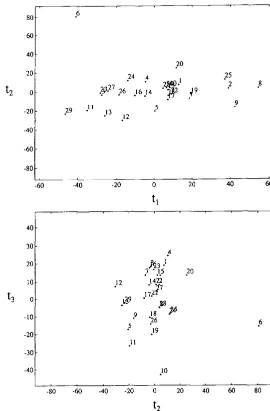
Fig. 8. Plots of  $t_1-t_2$  and  $t_2-t_3$  for 30 batches. Batch No. 6 is abnormal.
