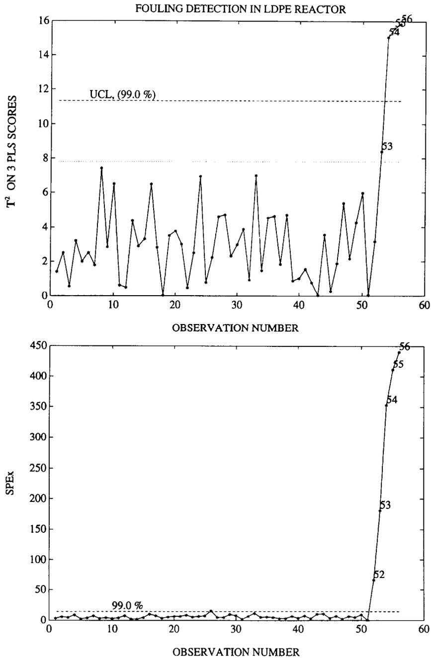
Fig. 4.  $T^2$  chart on three PLS scores and squared prediction error ( $SPE_x$ ) chart for monitoring the LDPE process. Points 52–56 denote a period where fouling occurred in the first zone of the reactor.
