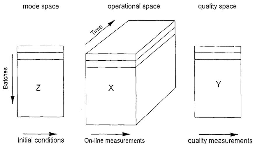
Fig. 7. Nature of batch data. The batch process is described by X, quality variables by Y and feed properties by Z.
