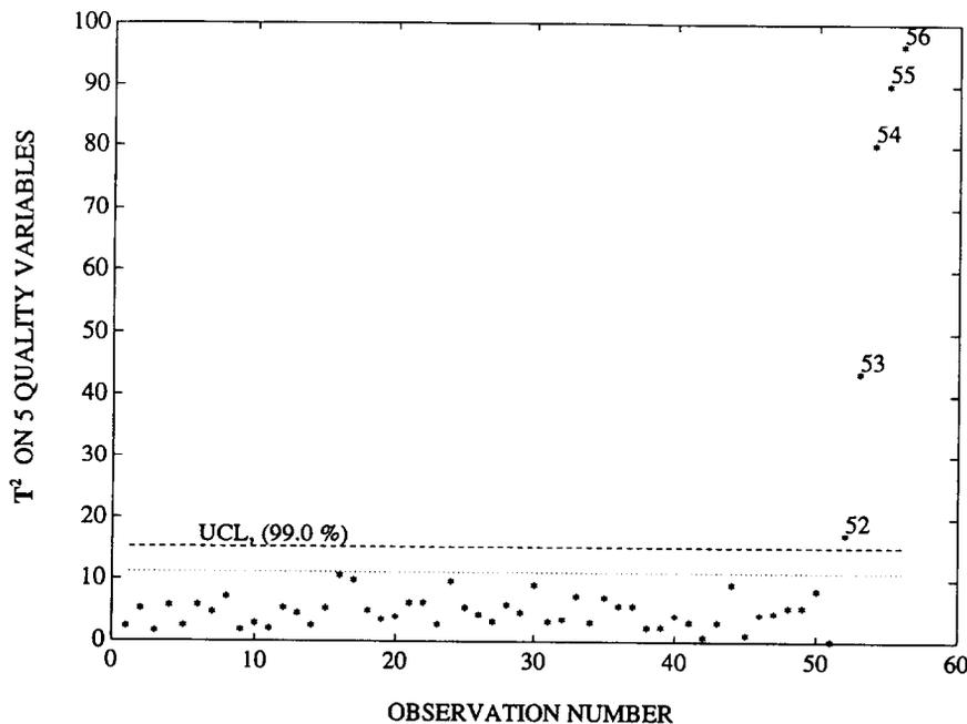
Fig. 2.  $T^2$  chart on five product properties of polyethylene.
