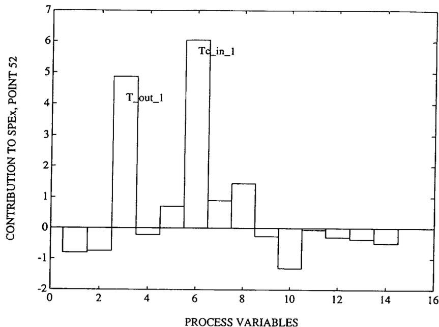
Fig. 5. Contribution plot showing the process variable contributions to the  $SPE_x$ , for point 52.
