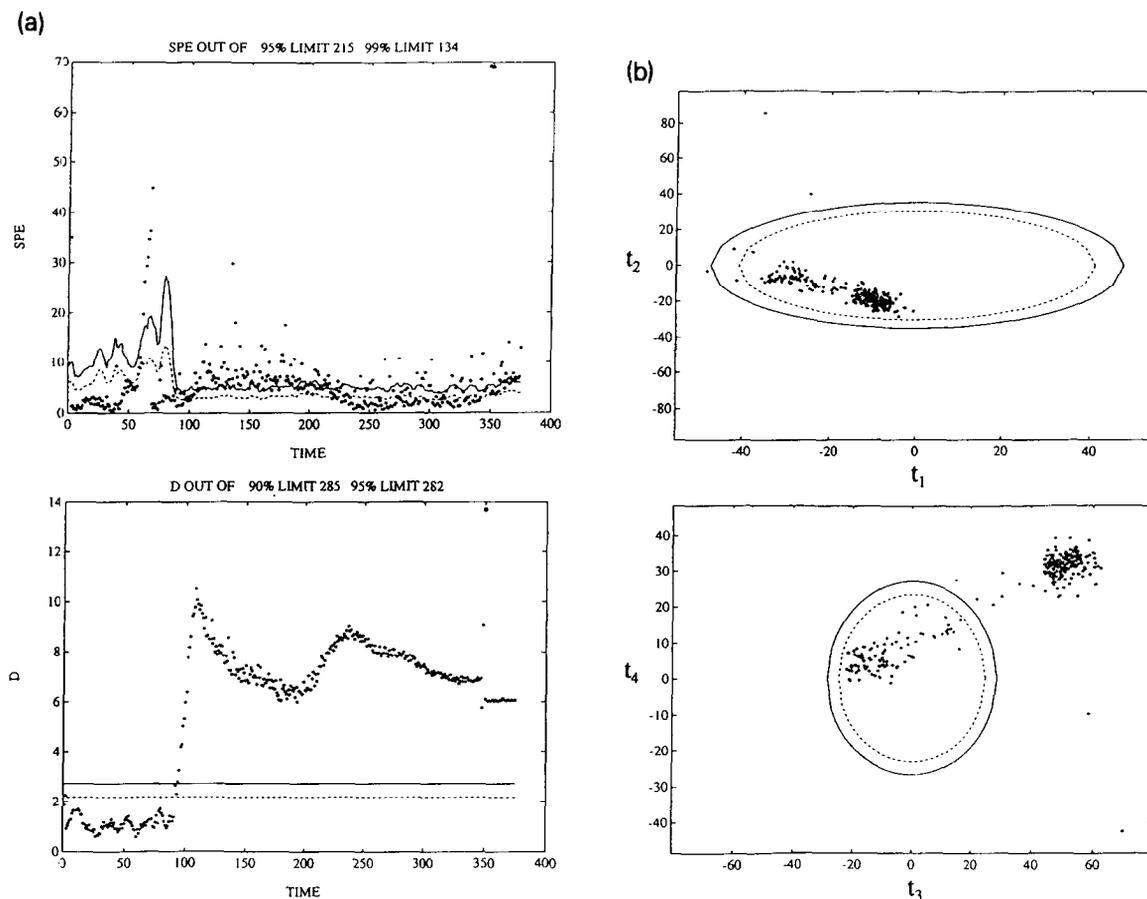
Fig. 10. Monitoring batch No. 6 (a bad batch). (a)  $SPE_x$  and  $D$  statistic. (b) Plots of  $t_1-t_2$  and  $t_3-t_4$  for the duration of the batch.
