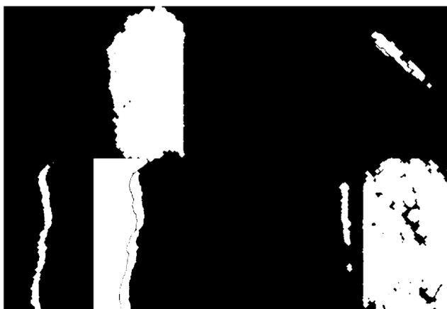
Fig. 4. Y-image mask of (0/1) discrimination areas. Note that by using a relevant background discrimination feature, it is possible to zoom in only on the true flaws present in the gridded calibration imagery, which have been designated white here.
