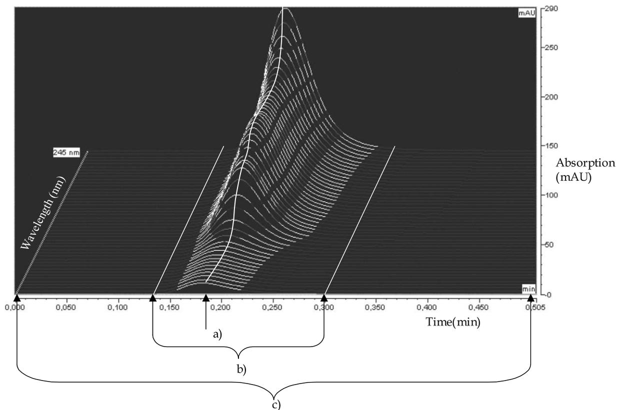
Fig. 2. Schematic image of the three approaches to export a representative UV spectrum from a collected DAD file. The 3D image is taken from Chromeleon version 6.11. (a) UV spectrum at spectrum maximum intensity time (SMIT), (b) average UV spectrum over sample peak, (c) average UV spectrum over whole DAD file.
