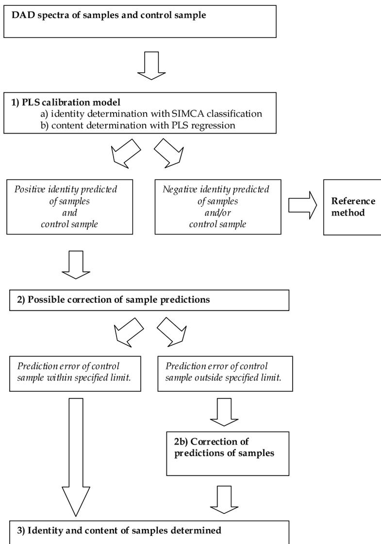
Fig. 4. Schematic diagram of the procedure for the identity and content determination with the DAD method using a control sample for estimation and correction of the prediction error.
